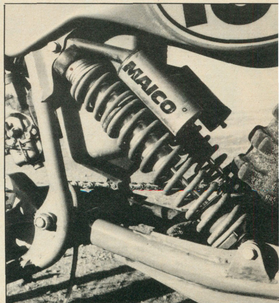
Corte Cossa supplies the piggyback shocks. They work well. The springs start out too stiff but sack their way down to soft.
